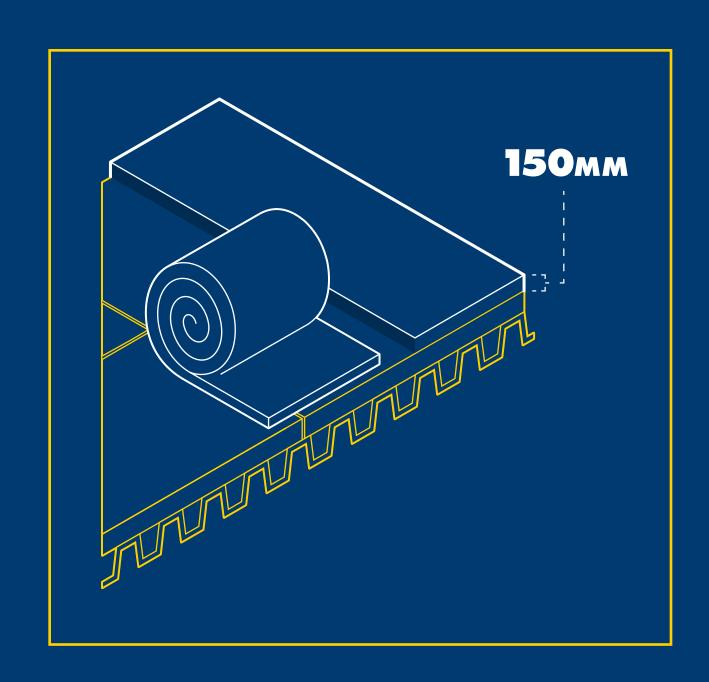
In sloping ceilings, you'll need to use 150mm insulation between rafters and 50mm underneath. For horizontal ceilings, you'll still need to use 400mm mineral/glass wool products.
